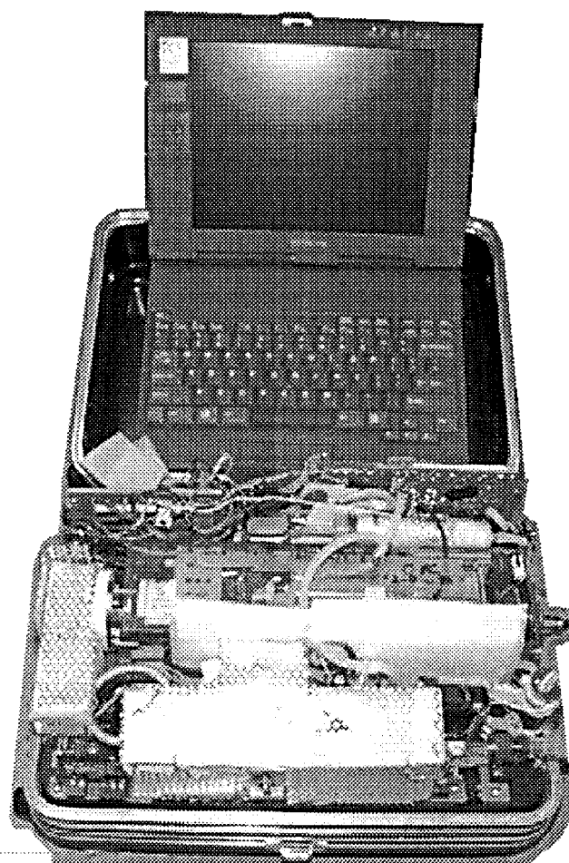
Figure 4 Gas chromatograph/ion mobility spectrometer for bacterial analysis.
